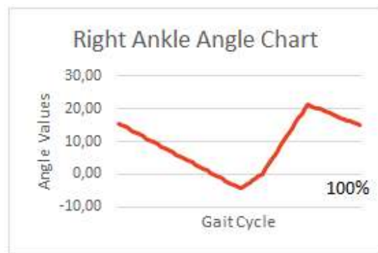
Fig. 14. Right Ankle Angles Result Of Biped Robot.
