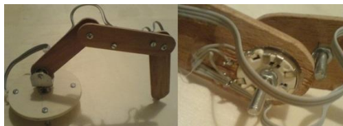
Fig. 1. Reference Arm and the situation of potentiometers placed on the joints
