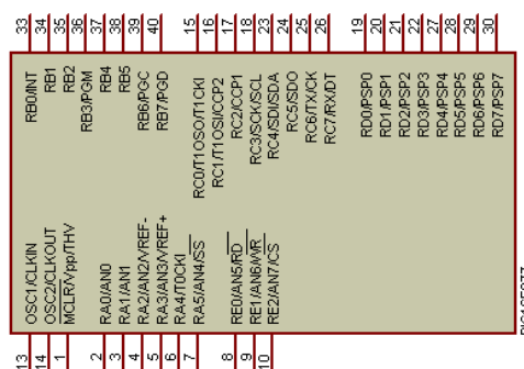
Figure-4, 16f877/a microcontroller's foot names.
