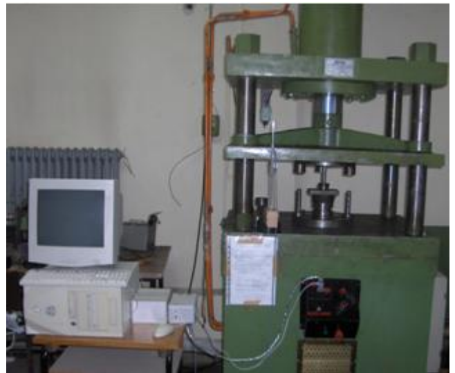
Fig. 11. View of Forging Press After becoming Computer controlled
