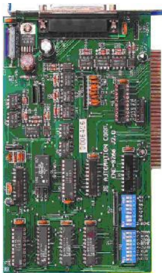
Fig. 6. View of the card which reads the Encoder value
