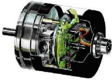
Fig. 4. The View of the Encoder which is reading the position information
