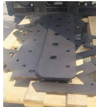
Figure 22. Design III - Cutting the plates with the laser-cutting device.
