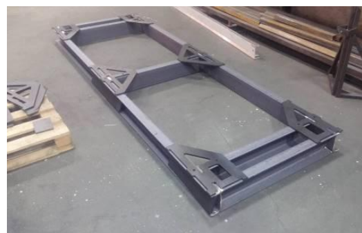
Figure 23. The welded joint of the structural system
