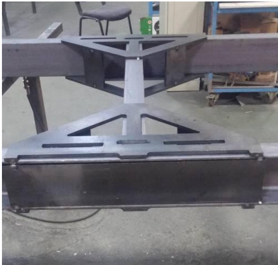
Figure 24. Mounting of the plates at the middle section of the carrier system
