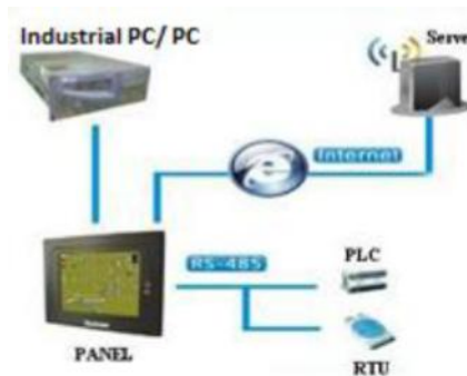
Fig. 8 The panel communication with other hardware
